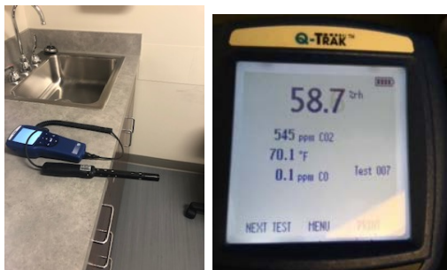
Picture 3: Q-TRAK CO 2 Measurement
